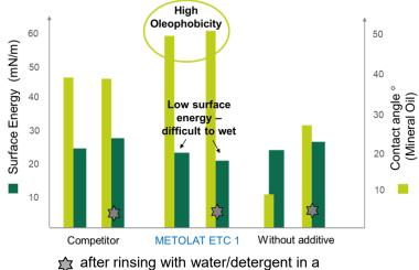
Low surface energy and high oil resistance (oleophobicity) achieved using METOLAT® ETC 1.
