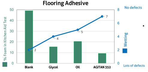
Minimal wetting defects vs. other defoamers while maintaining good foam control
