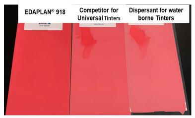
Improved resistance to flocculation in PR 254 in solvent-based alkyd.
