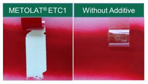
Resistance to spray paint and 'easy to remove' with tape
