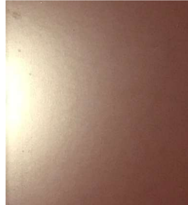
Customer paint with post-addition of 0.5% Additive A
