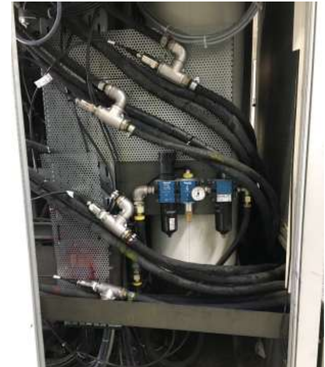
Inline integration of viscometers in coating circulation lines
