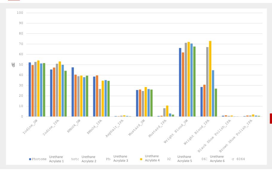
Formula samples were drawn down on white Leneta Charts with wire rod #3 (a film thickness of 13-16 microns) and two drawdowns (7x11 in) for each of the formula and cured in UV Fusion System at 25-30 ftm (945 mJ/cm²).
