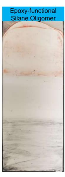
Epoxy-functional Silane Oligomer and Aminefunctional Silane Monomer both resisted staining more than coating made without silane
