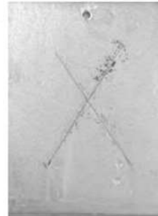
C: CrIII + silica passivate film on zinc
