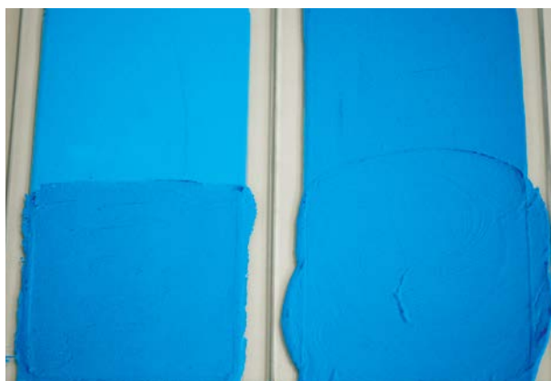
Figure 1 | Strong rub-out of PB15:3 in an emulsion paint No rub-out
