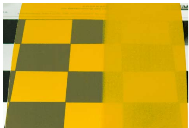
Figure 2 | Excellent transparency of PY 83 in a printing ink Bad transparency and formation of specks
