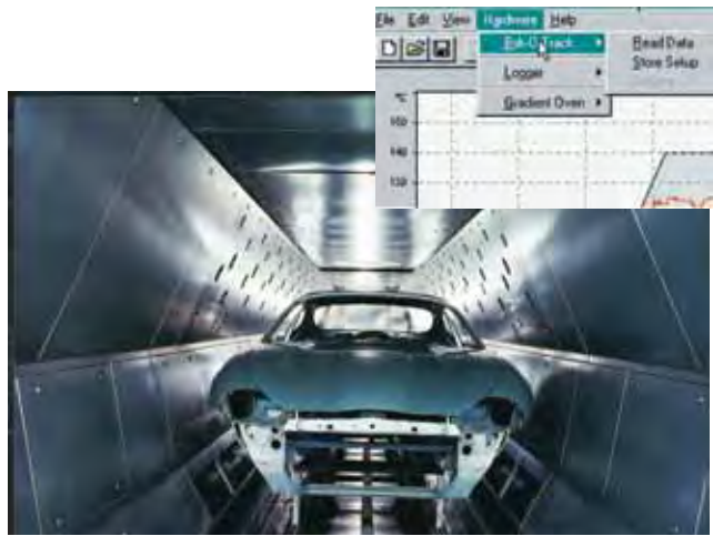
temp-gard collects temperature data in production oven.
