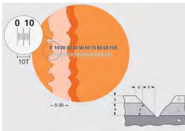
The thickness of multiple-layered coatings can be easily determined.
